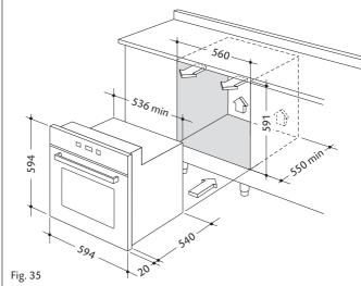
To ensure internal ventilation, aeration channels must be provided as illustrated in the figures 36 and 37.
